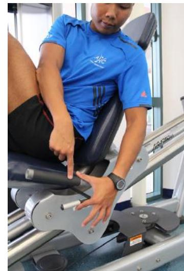
Pull the handle to adjust the seat. Move the seat forward so that the legs make a 90° angle when seated.
