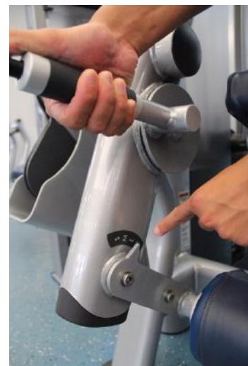
Pull the handle to adjust the leg pad. Position the pad just above the ankles.
