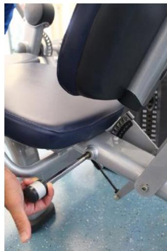
Pull the handle to adjust the backseat, so that the knee joint is aligned with the pivot point of the machine.
